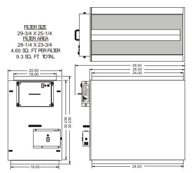
FILTER BOX WITH TWO FILTERS AND " STERILE SWEEP "
