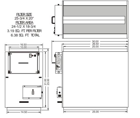
FILTER BOX WITH TWO FILTERS AND " STERILE SWEEP "
