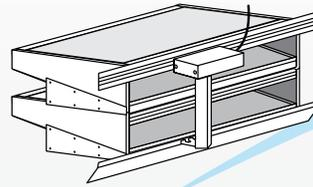
Power to Sterile Sweep Germicidal Units must go through an interlock switch on the chamber door. This will ensure the units are off when the chamber is entered.
