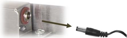
When unplugging the power cord from the air cleaner, care should be taken not to let the jack touch any metal or grounded surfaces. Even though the jack is shielded, it might still be possible for the central power insert to contact a grounded surface which could result in damage to the transformer or electronics.
